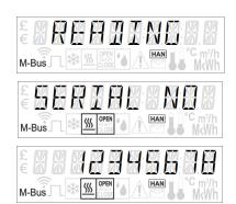
M-Bus icon will keep blinking until successful communication is established and will become stationary thereafter.
