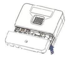
Figure 28: Opening the terminal cover
