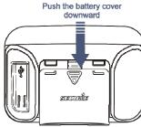
**Step 2:** Remove old batteries (if applicable) and place a pair of non-rechargeable AAA battery making sure of the correct polarity.
