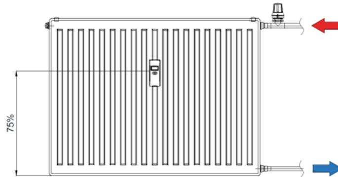
3. If it is not possible to install the allocator (heat sink) precisely in the middle of the radiator's width, move it closer to the side on which the heating medium supply pipe is located. Detailed information regarding this type of situation can be found in this document.
